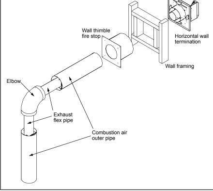
Figure 27. Horizontal Vent Termination
